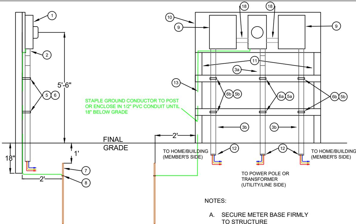
STAPLE GROUND CONDUCTOR TO POST OR ENCLOSE IN 1/2" PVC CONDUIT UNTIL 18" BELOW GRADE
