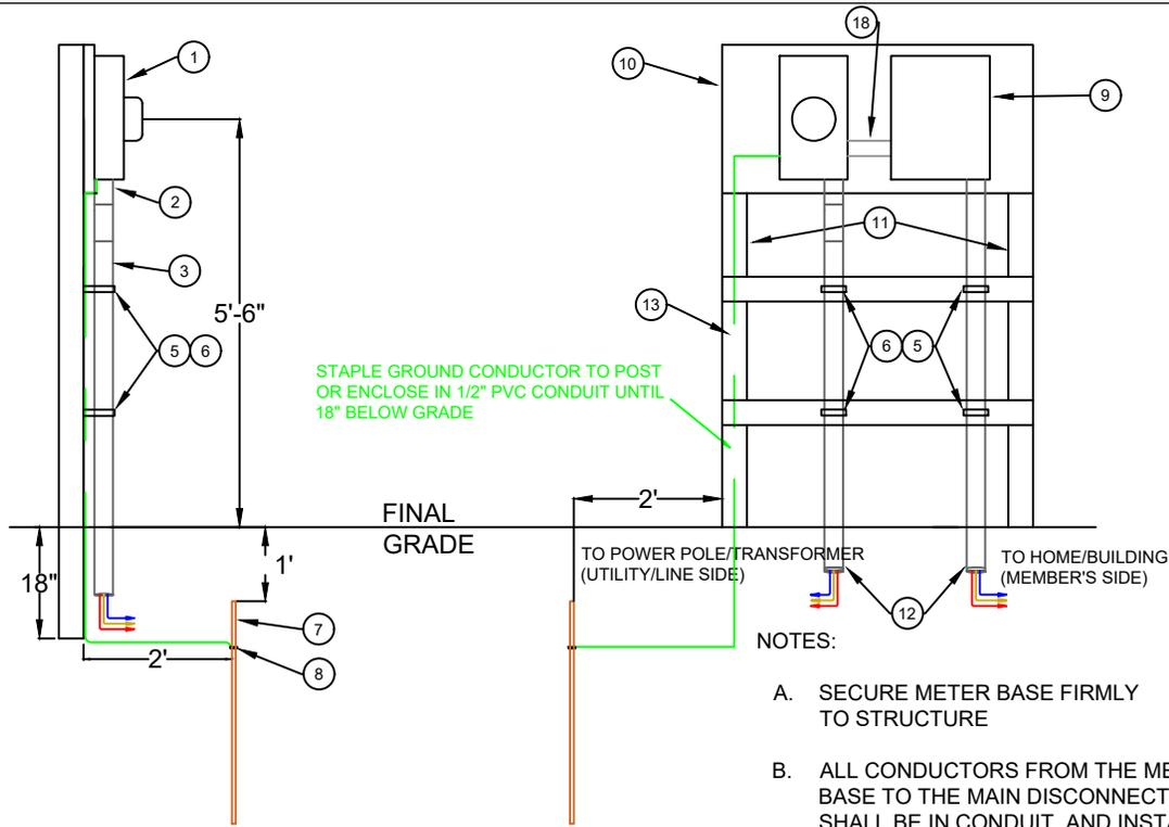
STAPLE GROUND CONDUCTOR TO POST OR ENCLOSE IN 1/2" PVC CONDUIT UNTIL 18" BELOW GRADE
