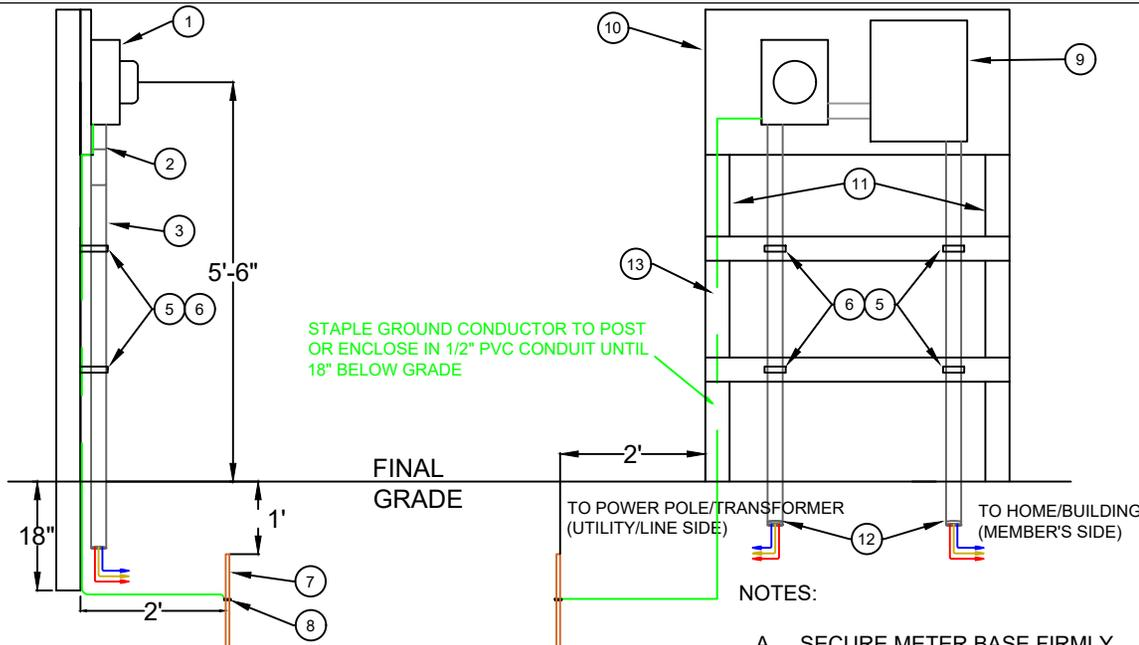
STAPLE GROUND CONDUCTOR TO POST OR ENCLOSE IN 1/2" PVC CONDUIT UNTIL 18" BELOW GRADE
